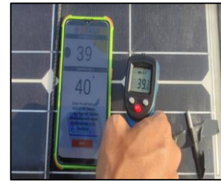
Figure 14. Temperature Verification Mobile Application Temperature Display Versus Temperature Measuring Device
