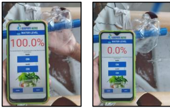
Figure 15. Testing the Distance Sensor
