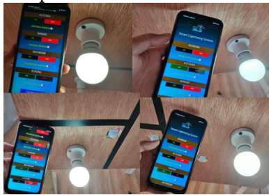
Figure 8: The SLS Android mobile application and Hardware test.
