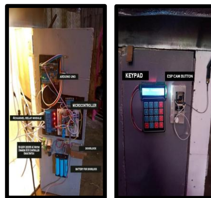
Figure 19. DOLAYT's IoT Hardware Components
