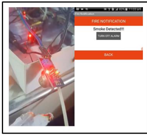
Figure 13. Testing of the MQ2 Smoke Sensor ( video reference:
