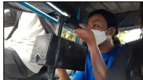
Figure 11: Vibration test in rough road and moving vehicle
