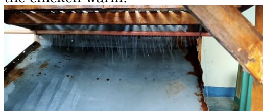
Figure 6. Testing the water washing the chicken's waste
